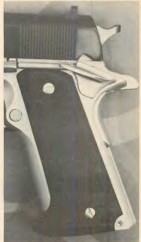
Rogers PPS stock design is such that removal and speed loading of magazine does not interfere with normal use.
